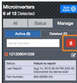
10. To add the new microinverter serial number, initiate a device scan by pressing the **Device Scan** button on the Envoy-S. The Envoy-S begins a 15-minute scan to identify all of the microinverters deployed at the site. The Microinverter Communications LED
